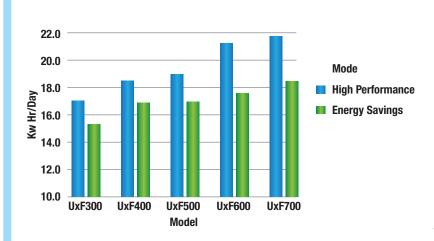
By controlling the temperature and time of the cycles, the energy savings cycle can save up to 15% while still offering tightly-controlled cabinet temperature and excellent door-opening recovery. The high-performance mode maintains the strictest cabinet temperature control.
